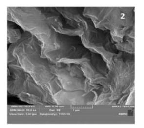
Figure 1. SEM micrograph of GNPs at x35k magnification
